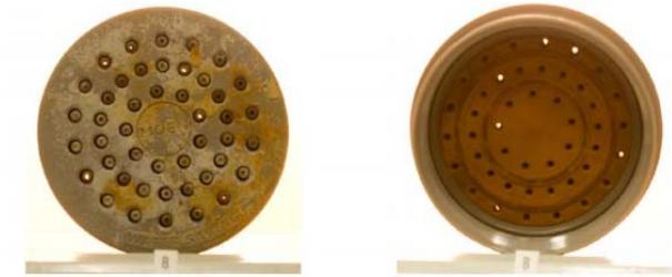
Top photo is of a showerhead after seven days of accelerated testing with soft water showing all 45 of 45 spray nozzles open. Bottom photo is of a showerhead after seven days of accelerated testing with hard water showing only 6 of 45 spray nozzles open.
